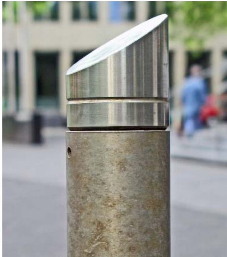
Slika 6: Vpliv soli na cestne stebričke. (vir: Houska, C. 2003. Deicing salt – recognizing the corrosion threath. Pittsburgh, TMR Consulting: 11 str.)
