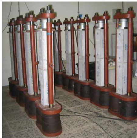
Slika 4.95: Prizme iz vlaknastega betona, vpete v jeklene jarme za preiskavo lezenja vlaknastega betona. Figure 4.95: Prism of fibre reinforced concrete fixed in steel frame for creep research of fibre reinforced concrete.
