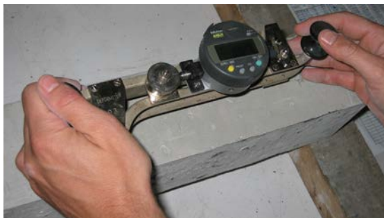
Slika 4.6: Meritev celotnega krčenja z nasadnim deformetrom Figure 4.6: Measurement of total shrinkage with inset deformeter
