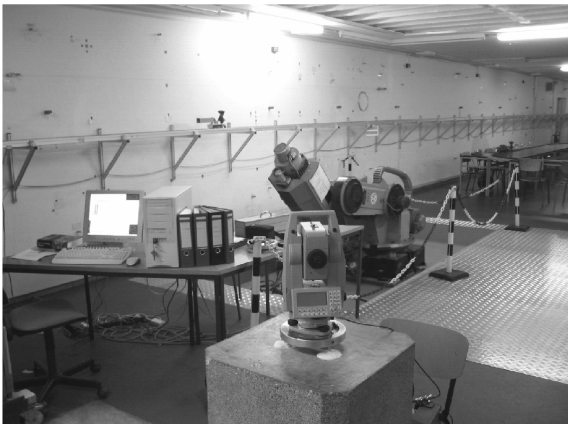
Slika 4.1: Geodetski laboratorij Katedre za geodezijo, TUM, z referenčno tirnico Figure 4.1: Geodetic laboratory at Chair for Geodesy, TUM, with reference trajectory
