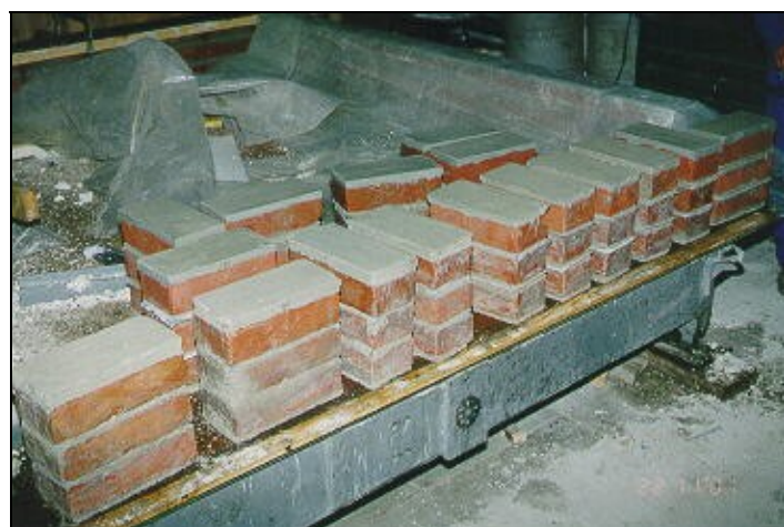
Slika 156: Zidani vzorci z vgrajeno vodoneprepustno zaporo Fig. 156: Masonry specimens with a damp-proof course
