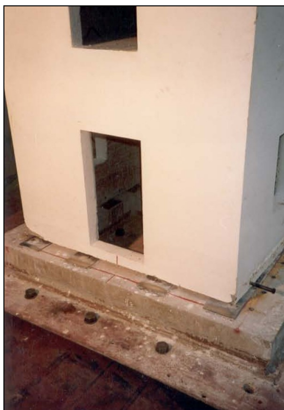
Slika 183: Zdrs modela po preiskavi Fig. 183: Model in the displaced position after the experiment
