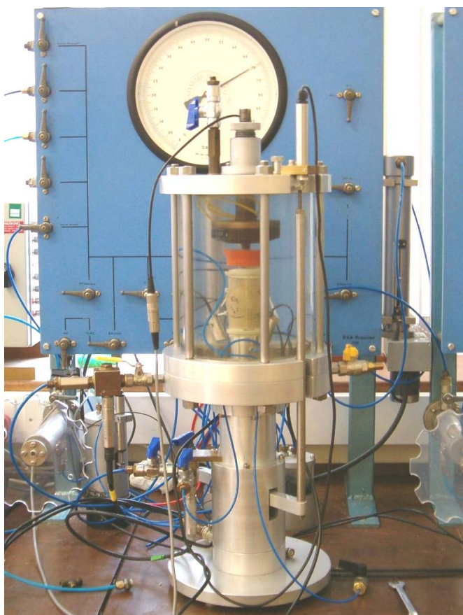
Slika 3.7: Triosni aparat B&W na Imperial Collegeu v Londonu. (foto: Carrera A.) Figure 3.7: Bishop and Wesley triaxial cell at Imperial College London. (photo by Carrera A.)
