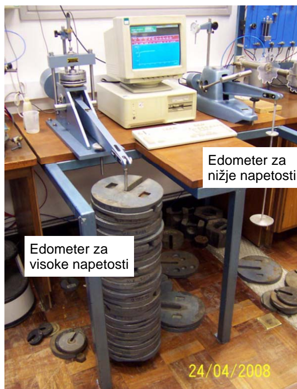
Slika 3.2: Edometra za visoke in nižje napetosti na Imperial Collegeu London Figure 3.2: Oedometer apparatuses for applying high and lower stresses at Imperial College London
