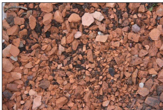
Slika 9: Streha 3 - substrat iz drobljene opeke (Vir: avtor) Figure 9: The roof 3 – crushed brick substate (Source: author)
