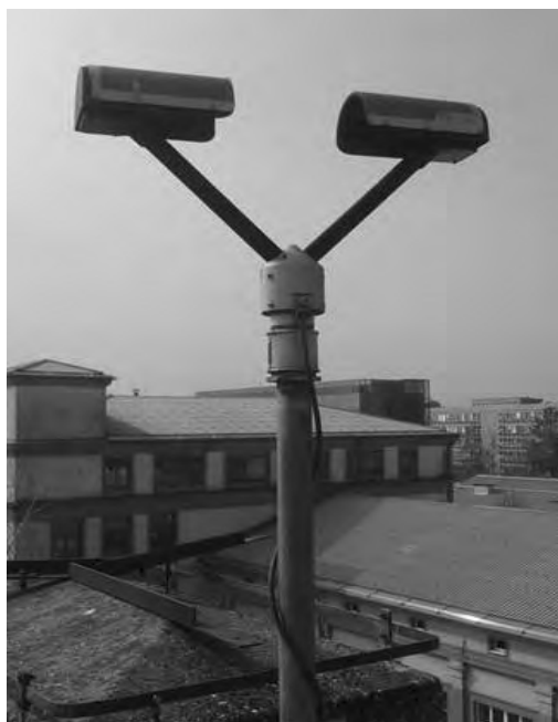
Slika 11: Disdrometer OTT Parsivel v Ljubljani Figure 11: Disdrometer OTT Parsivel in Ljubljana
