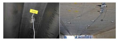
Figure 1: Strain gauges installed on a steel orthotropic-deck bridge (left), and a typical strain transducer set-up on a reinforced concrete bridge (right).
