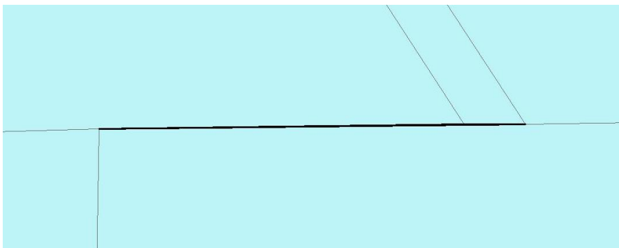
Slika 3: Primer topološke napake pri pravilu Must not overlap (OPN Šenčur, 2011)
