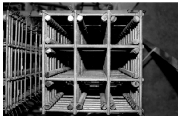
Fig. 2 (d)—20-bar reinforcing arrangement with 9-cell grids.
