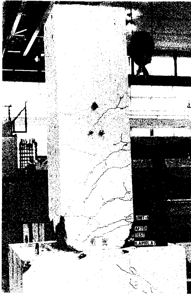
(a) Crack Patterns
