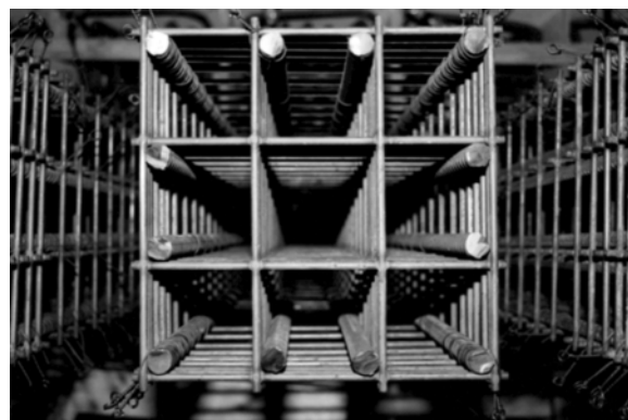
Fig. 2 (b)—12-bar reinforcement arrangement with 9-cell grids.
