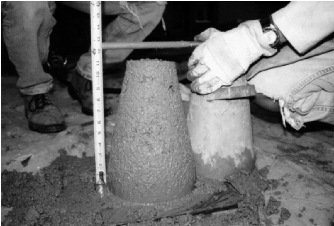
Figure A.27. Slump test for batch 2.
