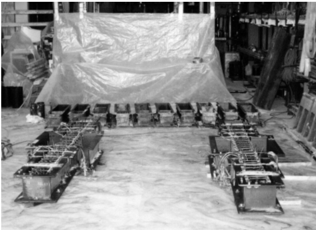
Figure A.20. Metal forms with cages and anchoring bolts in place, immediately before casting.
