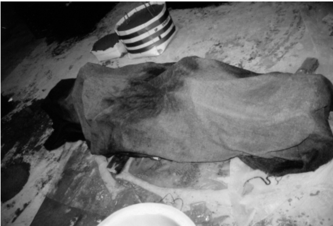
Figure A.28. Specimen covered with wet burlap during the curing period.
