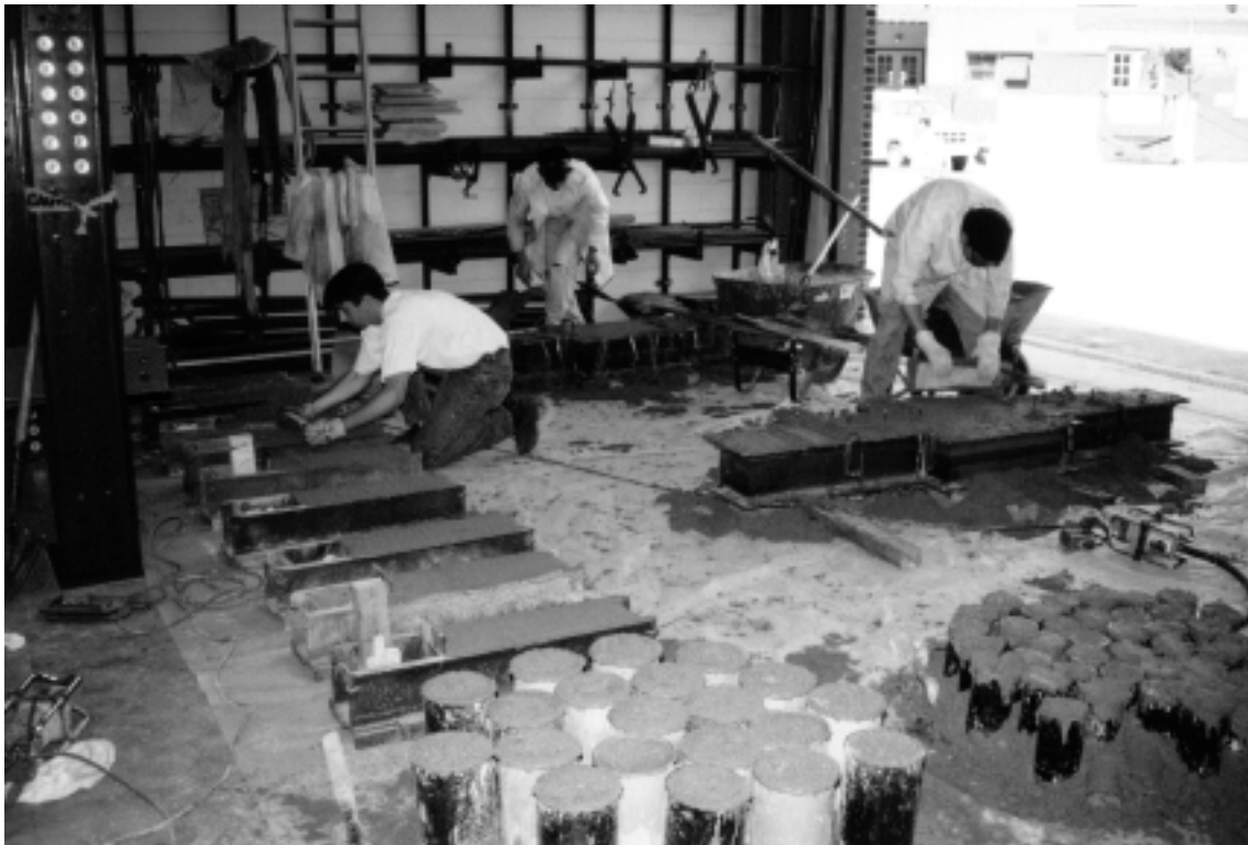
Figure A.25. Finishing the surfaces for specimens and flexure beams.
