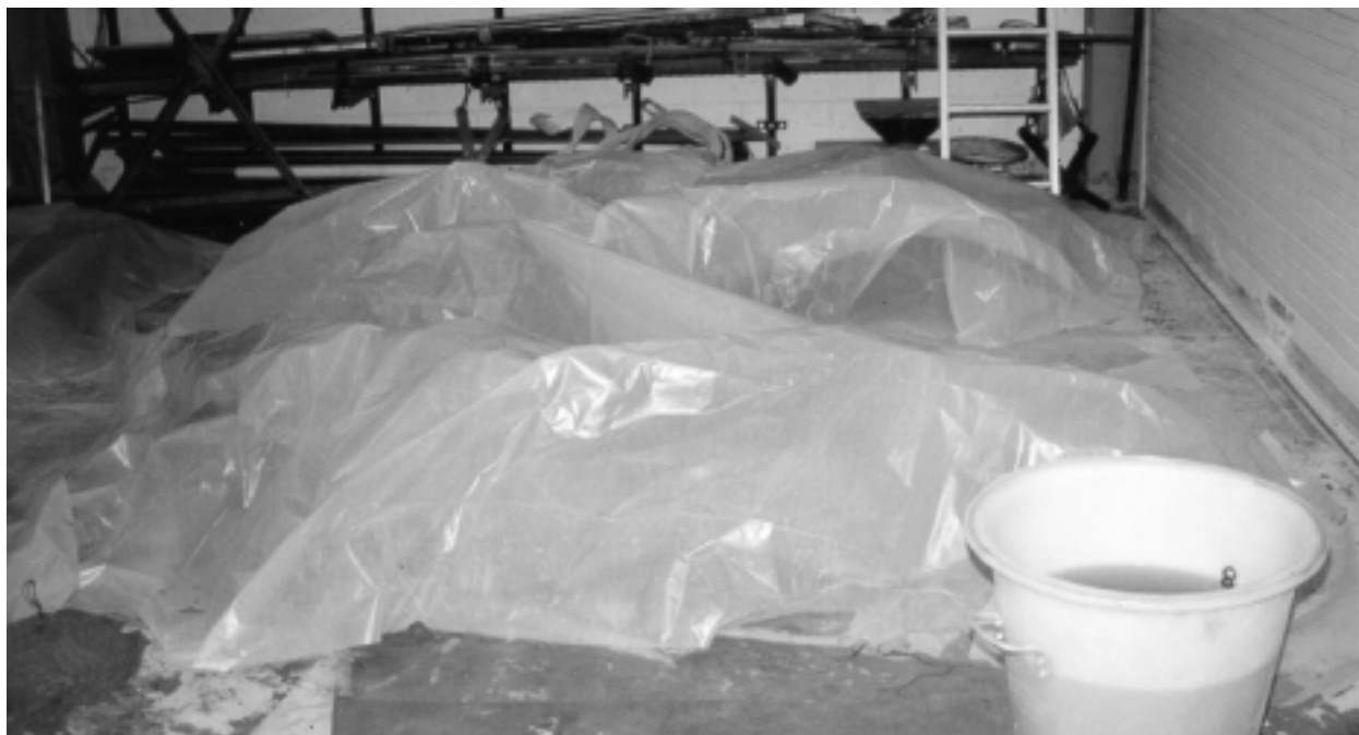
Figure A.29. Specimens, flexure beams and cylinders covered with wet burlap and plastic.
