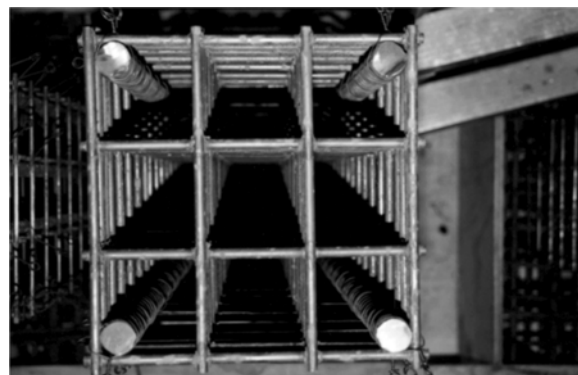
Fig. 2(c)—4-bar reinforcement arrangement with 9-cell grids.
