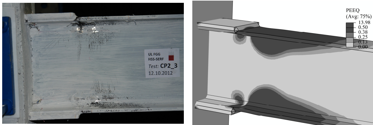
Fig. 127: Deformed shape of specimen CP2.3; comparison between the experiment and the simulation Slika 127: Deformacijska oblika preizkušanca CP2.3; primerjava med eksperimentom in simulacijo
