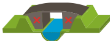
Slika 14: Odstranjevanje ovir pod mostovi (Dutch Water Program Room for the River, 2007)
