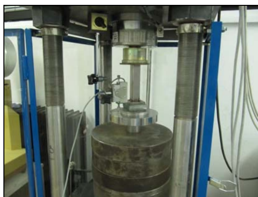
Figure 3.8: Compacting with hydraulic press and displacement measurements
