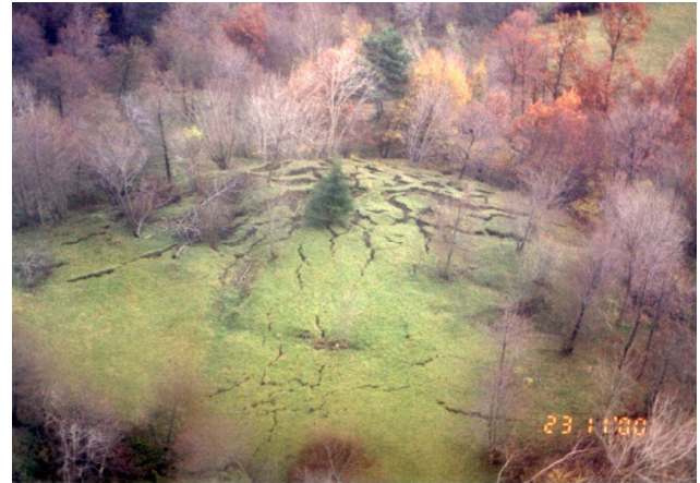
Fig. 5. The photo taken on 23 November 2000, at the location later on referred to as the “Lake of Mud” just before the vegetation was ripped off. Note the pronounced heave in the centre due to the pressure caused by the soil sliding.
