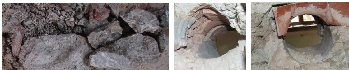
Slika 5.36: Jedro in globinske sonde, izvedene na zidu 3-AC2 Fig. 5.36: Core and in-depth probing at the wall 3-AC2
