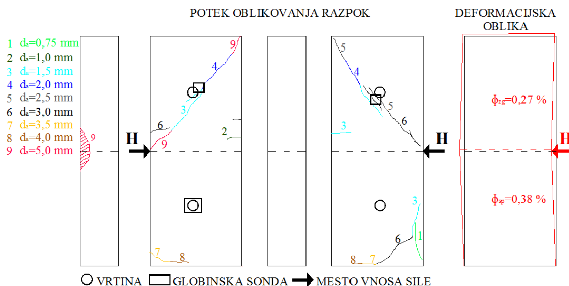
Slika 5.37: Oblikovanje razpok pri strižni preiskavi in deformacijska oblika zidu 4-C2 Fig. 5.37: Formation of cracks by shear test and deformation shape of wall 4-C2
