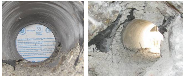
Slika 5.39: Vrtina in globinska sonda izvedena v spodnji polovici zidu 4-C2 Fig. 5.39: Borehole and in-depth probing at the lower half of the wall 4-C2
