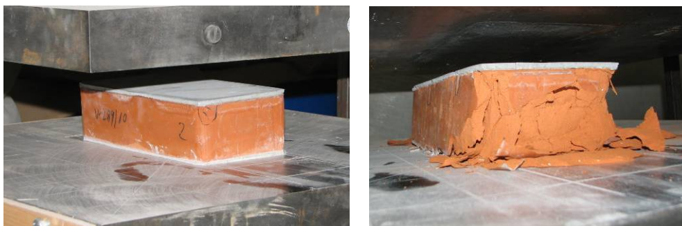
Slika 4.39: Opečni zidak pred (levo) in po preiskavi tlačne trdnosti (desno) Fig. 4.39: Brick unit before (left) and after compressive strength test (right)
