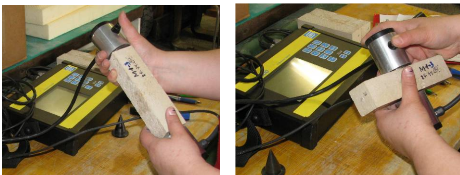
Slika 4.18: Meritve časa prehoda UZ na maltnih prizmah Fig. 4.18: Measurements of ultrasonics transition time through mortar prisms
