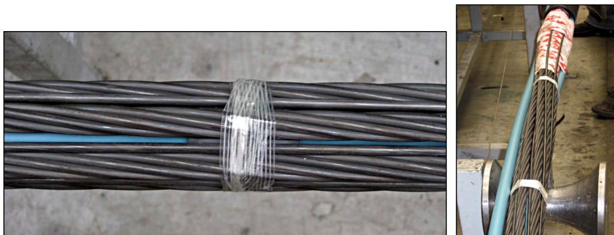
Slika 3.8: Detajla izdelave modificiranega prednapetega geotehničnega sidra RCP/D-K: potek žic med prameni (levo), zgornji del veznega dela sidra RCP/D-K s tesnilnim stikom (desno). Figure 3.8: Details of production of a modified prestressed ground anchor (type RCP/D-K): positioning of wires between strands (left), upper part of bond length of the anchor RCP/D-K with packing connection (right).
