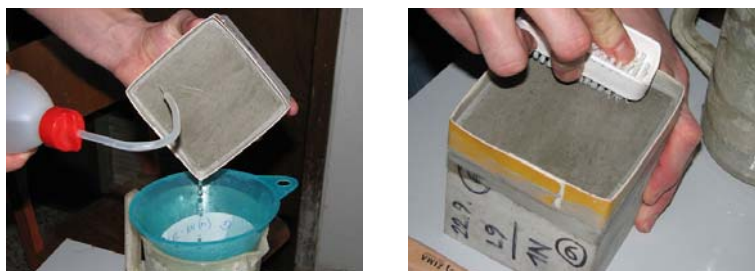
Slika 5.6: Odstranjevanje odlučenega materiala pri OSMO preiskavi s curkom vode (levo) ali s krtačko (desno) Fig. 5.6: Removal of scaled material in the salt frost scaling test with a jet of water (left) or with a brush (right)
