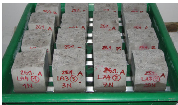
Slika 5.34: Rezultati testa vodovpojnosti betona s kapilarnim srkom po nekaj dneh Fig. 5.34: Results of concrete water absorption test after few days
