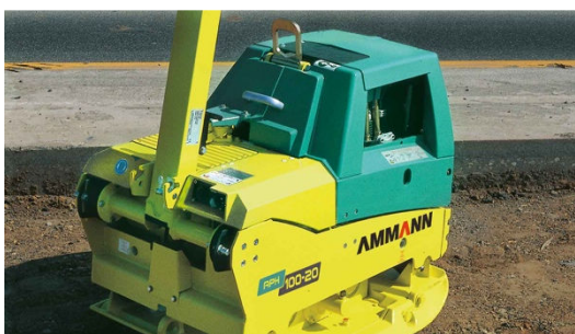
Slika 32 Vibracijska plošča (Vir: lastni arhiv) Figure 32 Hydrostatic vibratory plate (Source: personal archive)
