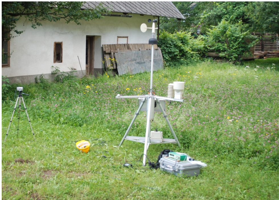
Slika 20 Meritve meteoroloških parametrov s prenosno vremensko postajo Vaisala MAWS201 (Vir: lastni arhiv) Figure 20 Measurements of meteorological parameters with portable weather station Vaisala MAWS201 (Source: personal archive)
