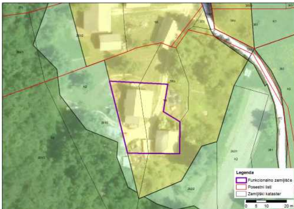
Slika 53: Dolo eno funkcionalno zemljiš e na podlagi sekundarnih in dopolnilnih virov za obravnavan primer 3 (Geodetska uprava RS in MO Novo mesto) Figure 53: Allocated functional site based on secondary and complementary sources for the studied case 3 (The Surveying and Mapping Authority of RS ang Municipality of Novo mesto)
