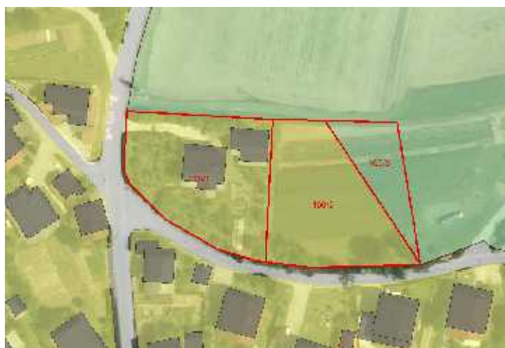
Slika 62: Oblikovanje parcel po predlaganih pravilih za formiranje parcel v zemljiškem katastru (Geodetska uprava RS in MO Novo mesto) Figure 62: Plot formation based on the proposed rules of plot forming in land cadastre (The Surveying and Mapping Authority of RS ang Municipality of Novo mesto)
