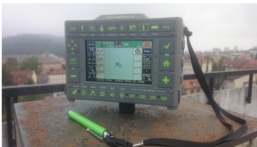
Slika 1: Instrument JAVAD TRIUMPH-LS
