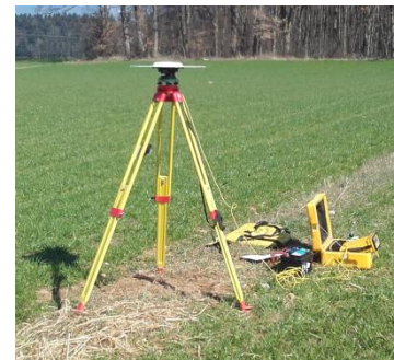
Slika 7: Instrument Trimble 4000SSi z anteno Trimble Compact L1/L2 with ground plane
