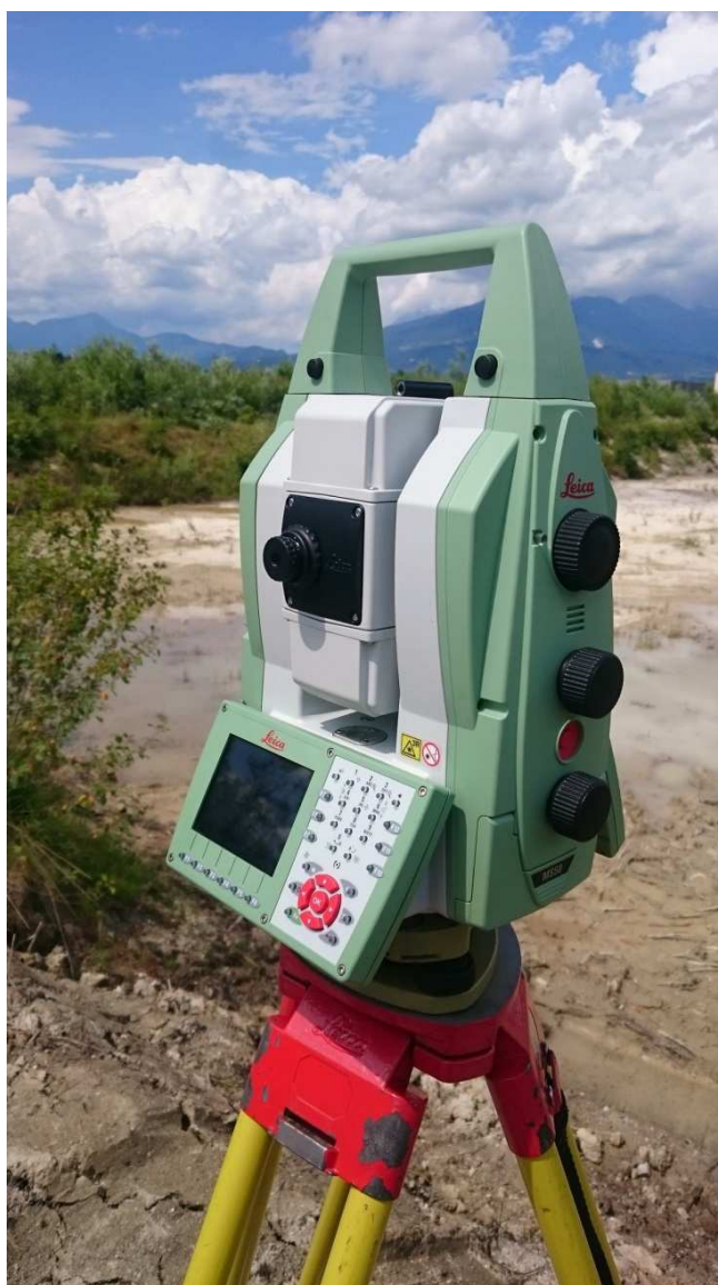
Slika 4: Tahimeter Leica Nova Multistation MS50
