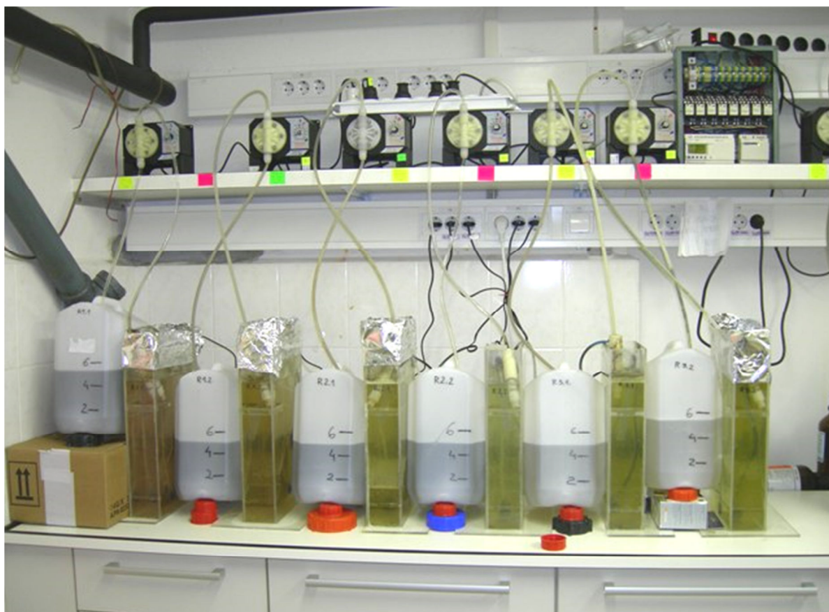
Figure 2: Pilot wastewater treatment plant showing bioreactors, plastic tanks with feeding mixture and pulse pumps.
