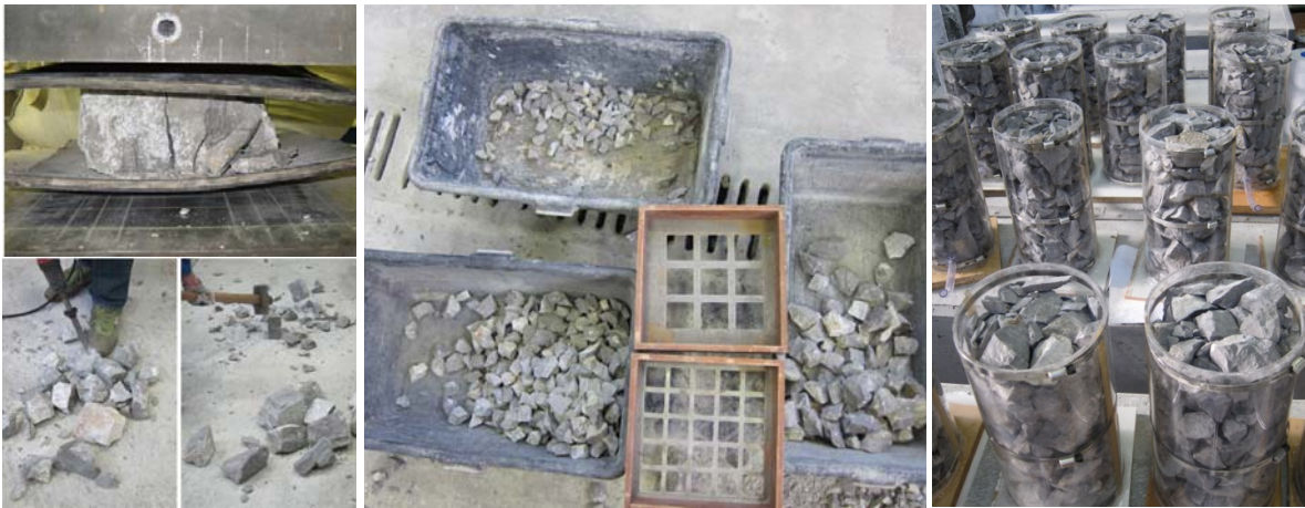
Figure 4.3: Crushing of stone blocks first by hydraulic jack, then by drilling and finally with hammer, sieved stone rubble and cylinders before grout injecting
