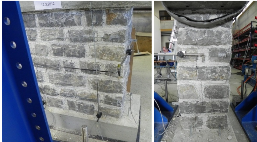
Figure 3.16: Damage of the wallette with header stones after test TP-1 Slika 3.16: Poškodbe na povezanem zidku po testu TP-1
