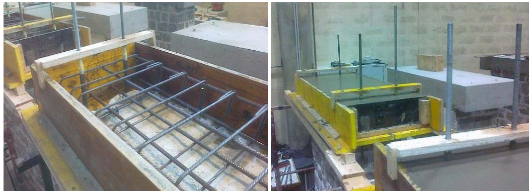
Figure 3.3: Cast with steel reinforcement for the upper concrete block [43]
