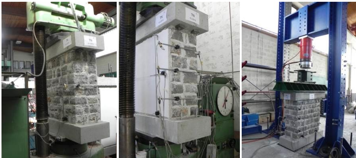
Figure 3.10: Test setup for the first test in the 5000 kN hydraulic jack (left two) and the following with 2500 kN capacity (right)
