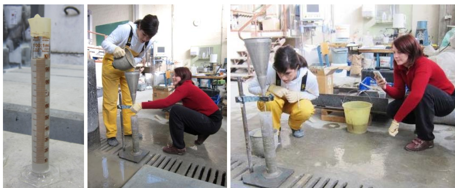
Figure 4.2: Bleeding test (left) and fluidity test (middle and right) Slika 4.2: Preizkus izločanja vode (levo) in pretočnosti (na sredini in desno)
