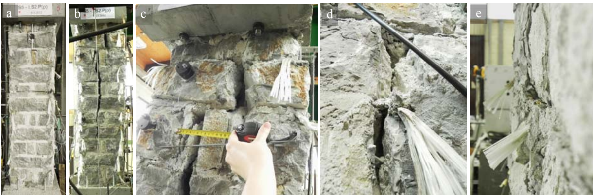
Figure 5.16: Leaf separation with toe-crushing (a-c), damage of the transversal connections (d, e) of the wall after test S5 - I.S2.P(p) Slika 5.16: Razpoka (vrzel) med slojema ter zdrobljena peta (a-c), poškodovanost prečnih povezav (d, e) zidu po testu S5 - I.S2.P(p)
