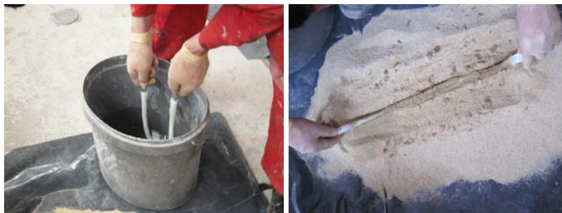
Figure 4.16: Impregnating the cord with an epoxy resin (left) and coating the cords in quartz sand (right) Slika 4.16: Namakanje vrvice v epoksi smolo (levo) in valjanje vrvice v kremenčevem pesku (desno)
