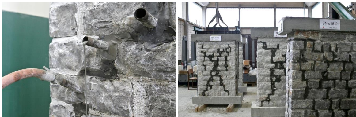
Slika 8.13: Injektiranje zidov z iztekanjem injekcijske mase in zidovi po injektiranju Figure 8.13: Grouting of walls along the cracks with grout leakage and specimens after grouting
