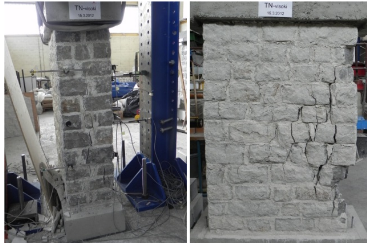
Figure 3.19: Damage of the wall without through stones after test TN-visoki Slika 3.19: Poškodbe na nepovezanem zidu po testu TN-visoki
