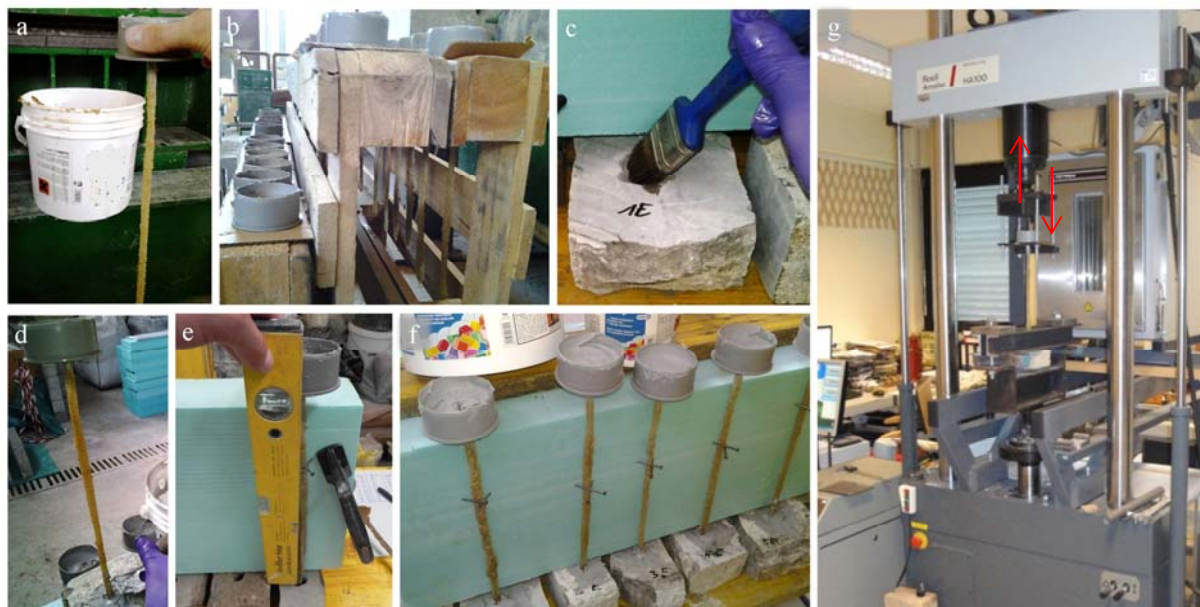
Figure 4.10: Preparation of the samples for the stone-mortar-cord junction tests: a) with epoxy resin impregnated cord coated with quartz sand and mounted with epoxy mortar in a PVC cap, b) hardening of the cords, c) application of the primer (in case of epoxy mortar), d) installing the cord with selected mortar, e) vertical positioning of the cord, f) hardening of the samples and g) test setup (adopted from [255] )
