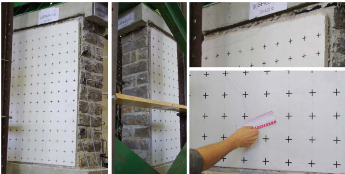
Figure 3.73: Detachment of the plaster and horizontal and diagonal crack on the plaster at test 1.2 - SPk-5-1 (7.5) Slika 3.73: Odstopanje ometa in horizontalna ter diagonalna razpoka na ometu pri testu 1.2 - SPk-5-1 (7.5)
