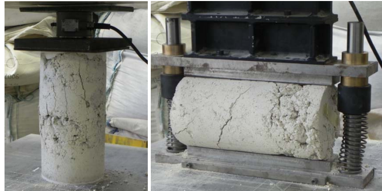
Figure 3.8: Compressive (left) and splitting tensile strength (right) test of the cylinder core sample Slika 3.8: Tlačni (levo) in cepilni (desno) preizkus valjastega vzorca jedra
