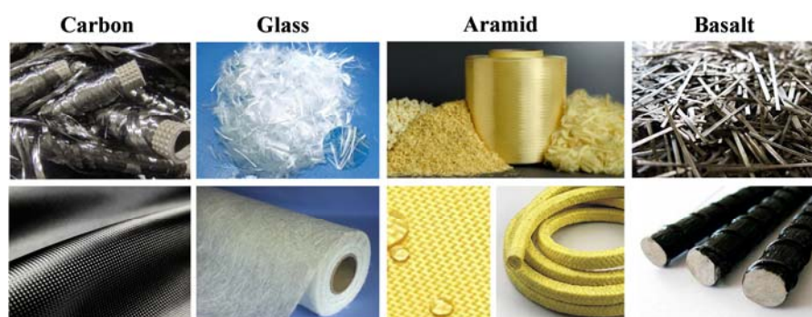
Figure 2.27: Carbon fibre tow ( http://www.rockwestcomposites.com/products/10015-d ) and fabric ( http://www.sailingscuttlebutt.com/2013/10/17/addressing-environmental-impact-carbon-fiber/ ), glass fibres ( http://image.made-in-china.com/4f0j00BvraECiGRWzQ/Glassfiber.jpg ) and mat ( http://shop.hp-textiles.com/shop/product_info.php/language/en/info/p98_hp-mp300e---textile-glass-mat.html ), aramid fibres and filament (upper photo) and fabric ( http://kevlar-fiber.com/ ), braided aramid ( http://www.directindustry.com/prod/aw-chesterton-company/aramid-braided-packing-17469-526554.html ), basalt fibres ( http://www.technobasalt.com/i/products/439_241/GLY57W8x.jpg ) and rods ( http://www.directindustry.com/prod/technobasalt-invest-llc/basalt-fiber-reinforced-polymer-bar-65468-1007959.html )
