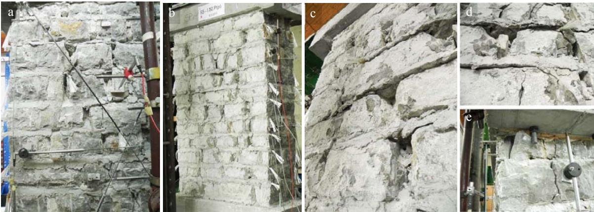
Figure 5.15: Crack pattern on the wall (a, b) with cord detachment (c, d) and toe crushing (e) after test S5 - I.S2.P(p) Slika 5.15: Razpokanost zidu (a, b) z odstopanjem vrvice (c, d) in zdrobljeno peto (e) po testu S5 - I.S2.P(p)
