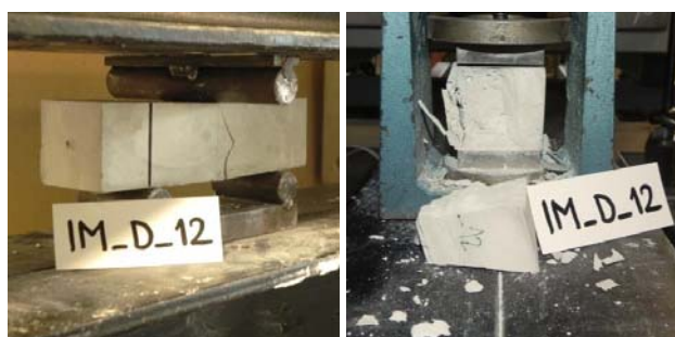
Figure 4.5: Flexural (left) and compressive (right) test on the mortar prisms [251] Slika 4.5: Upogibni (levo) in tlačni (desno) preizkus maltne prizme [251]
