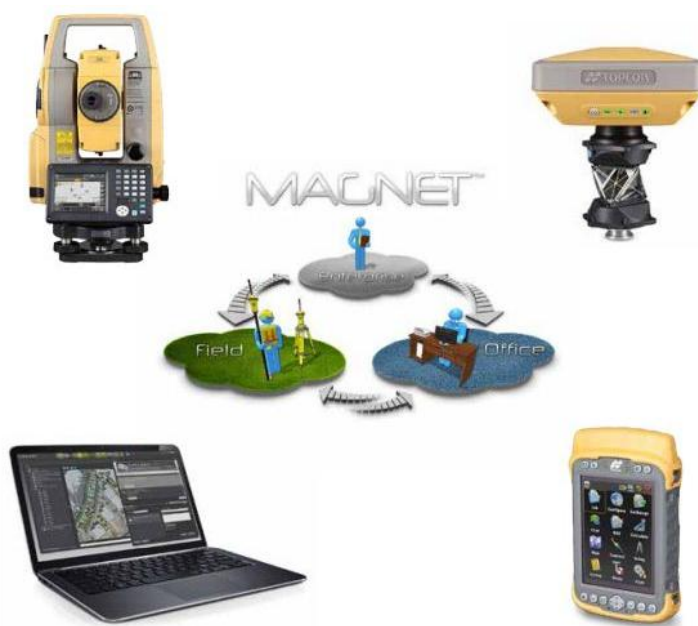
Slika 10: Prikaz komponent sistema Topcon Hybrid positioning (vir: Topcon Hybrid Positioning, 2013)
