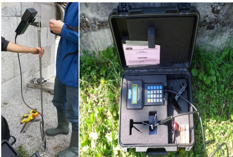
Slika 19: Priprava instrumenta Flow Tracker Handheld ADV.
