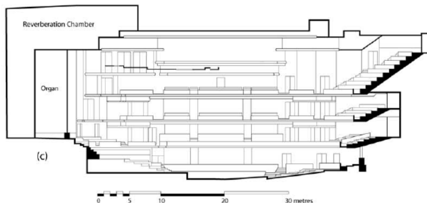
Slika 6: Odmevnica (reverberation chamber) [5]
