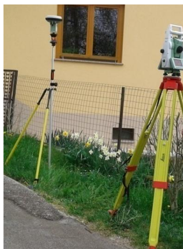
Slika 12: GNSS instrument in tahimeter sistema Leica Smartpole.
