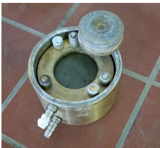
Slika 16: Vzorec temeljnih tal, premera 50 mm in višine 20 mm, vgrajen v tog kovinski obroč edometrskе celice Figure 16: Foundation soil sample (diameter 50 mm, height 20 mm), put into Oedometer ring
