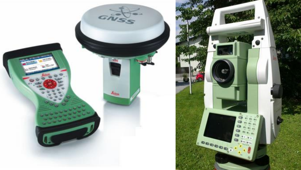
Slika 26: GNSS sprejemnik Leica Viva GS15 in instrument Leica TCRP 1201 (vir: Surveying Equipment, 2015 in Fröhlich, 2013)
