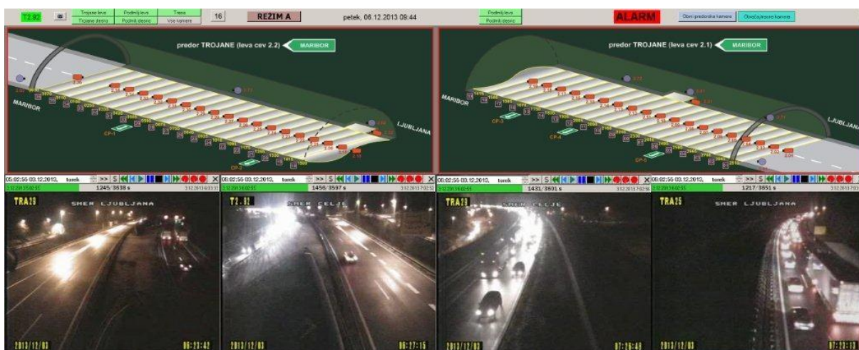
Slika 6-16: Nastanek zastoja pred predorom zaradi okvare tovornega vozila v predoru Trojane Figure 6-16: Congestion in front of the tunnel due to heavy vehicle breakdown in tunnel Trojane
