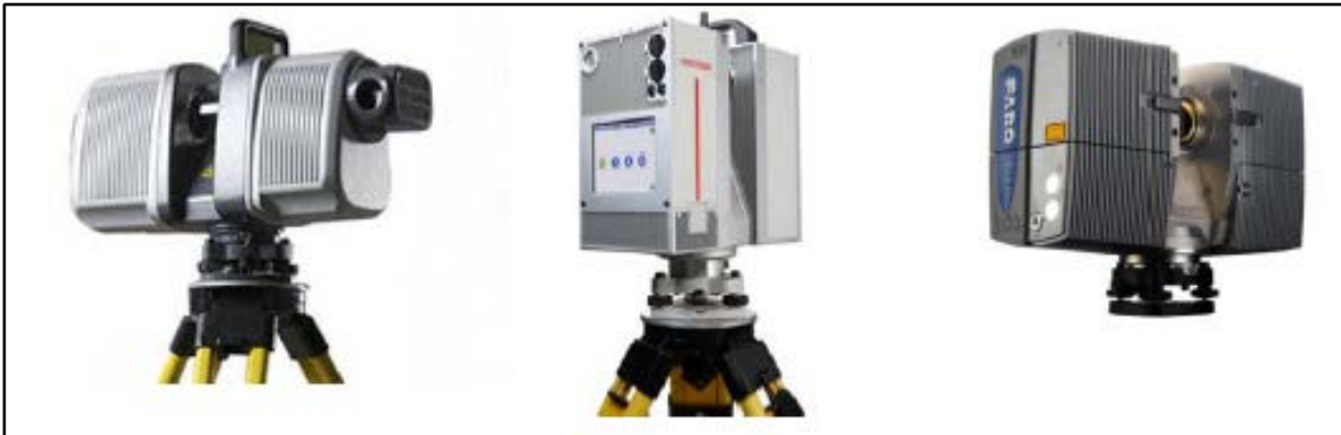
Slika 3: Fazni skenerji (Trimble CX Scanner, Leica HDS 7000, Faro Focus 3D) (Vir: Kogoj, 2013-2014).
