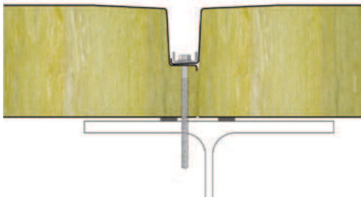
Fig. 2.9: Consequences of excessively tightened screw
