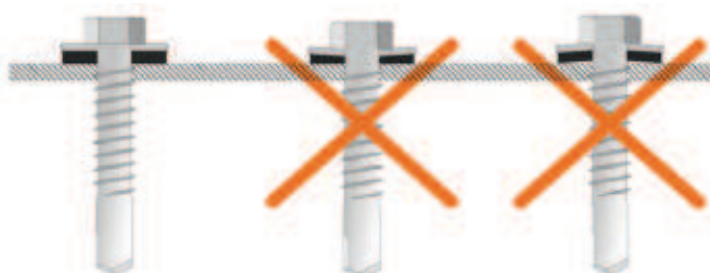
Fig. 2.10: Proper and improper fixing of screws
