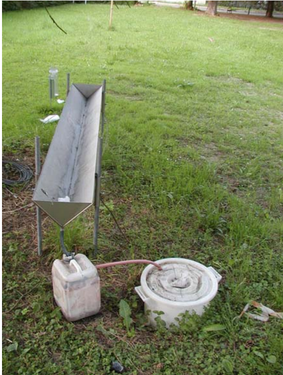
Slika 3. Korita in totalizator za merjenje prepuščenih padavin / Throughfall measurement with gutter and totalisator.
