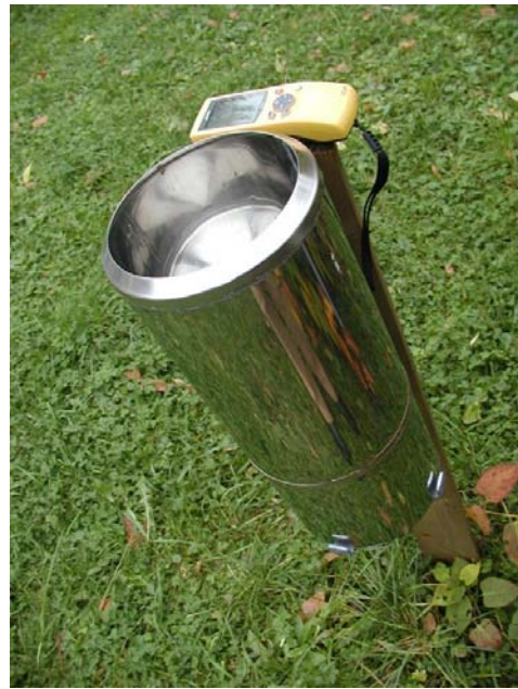
Slika 2. Ombrograf Onset RG2-M in Helmanov dežemer za merjenje padavin na prostem / Onset RG2-M and Helman rain gauge for measuring gross precipitation.
