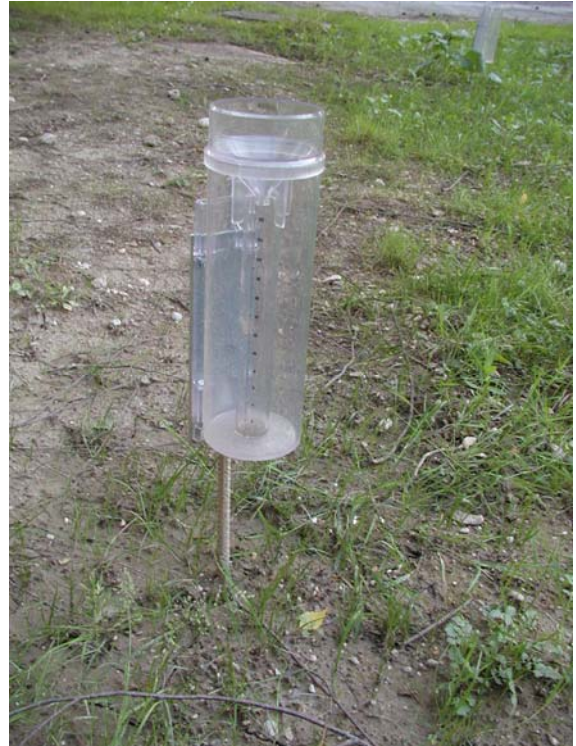
Slika 3. Korita in totalizator za merjenje prepuščenih padavin / Throughfall measurement with gutter and totalisator.
