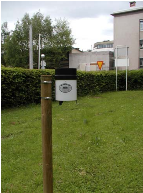
Slika 2. Ombrograf Onset RG2-M in Helmanov dežemer za merjenje padavin na prostem / Onset RG2-M and Helman rain gauge for measuring gross precipitation.
