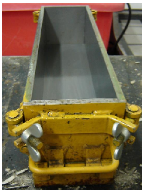
Slika 20: Kalup prizme 100x100x400 mm.
