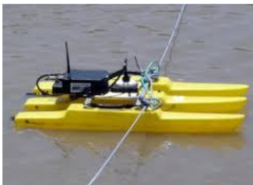
Slika 33: Katamaran z instrumentom SonTek ADP (Sontek, 2013)
