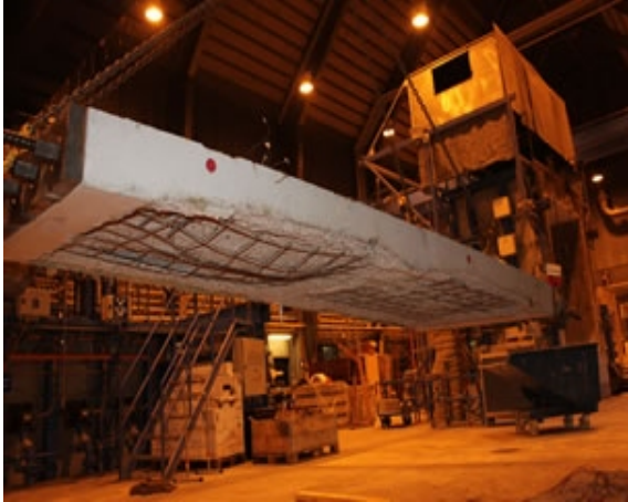
Slika 2.4: Posledice luščenja betona po požarnih testih (Fire spalling ..., 2013, Tunnel fire ..., 2013). Figure 2.4: Spalling damage of concrete after fire tests (Fire spalling ..., 2013, Tunnel fire ..., 2013).
