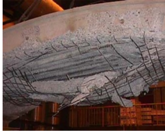
Slika 2.4: Posledice luščenja betona po požarnih testih (Fire spalling ..., 2013, Tunnel fire ..., 2013). Figure 2.4: Spalling damage of concrete after fire tests (Fire spalling ..., 2013, Tunnel fire ..., 2013).
