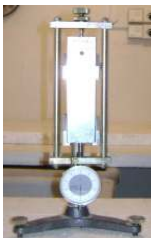
Slika 36: Graff-Kaufmanov deformeter (Golob, 2007)
