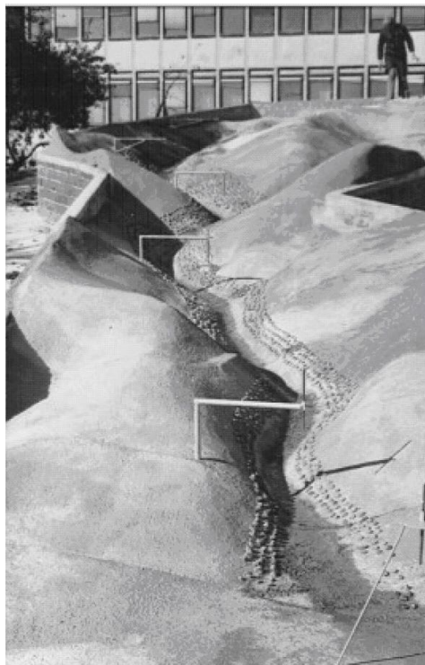
Fig. 1. Photo of physical model of south valley with installed gauges
