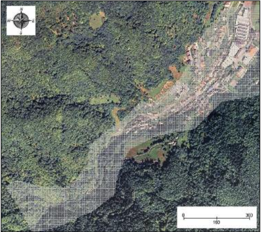
Figure 5: The computing grid 5m×5m for the Hrenovec torrent and the village of Kropa.
