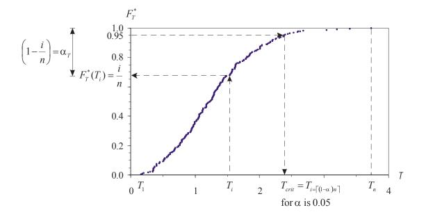
**Figure 1:** Empirical cumulative distribution function of the test statistic  $T = d / \sigma_d$
