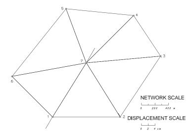
Figure 2: Test network and displacements
