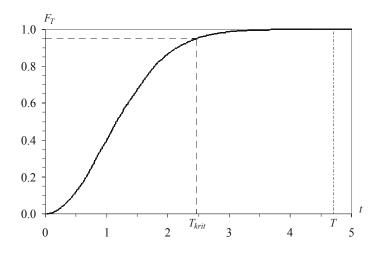
**Figure 3: D**istribution function of test statistic for Point 2:  $T = d / \sigma_d = 4.724$
