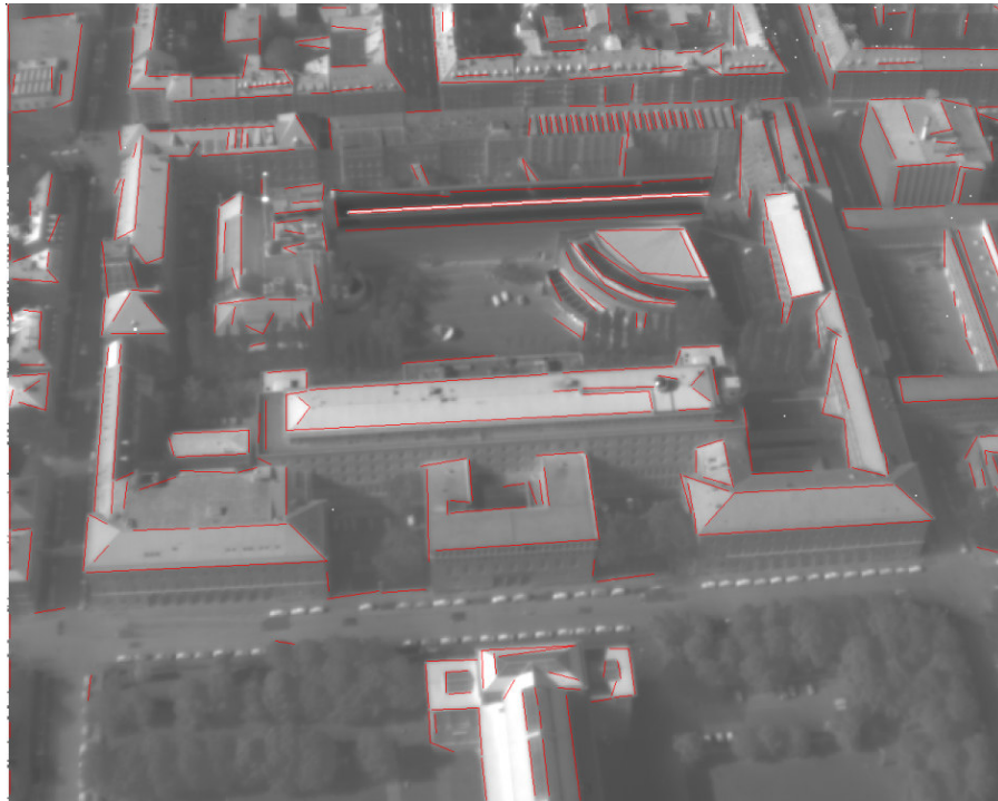
Figure 14: Extracted straight edges (red). Input variables are input image: 13200, filter size: 9 \times 9 px, minAmp: 18 px, maxDist: 5 px, minLength: 10 px
