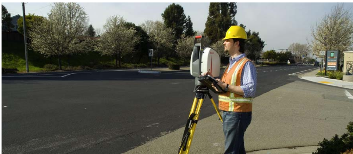
Slika 2.1: Laserski skener na terenu - Leica Scan Station 2 (Leica Geosystems, 2009)
