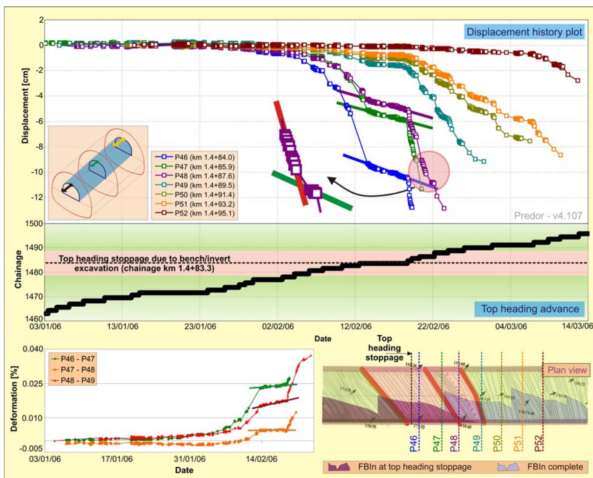
Figure 5-37. Longitudinal displacement pattern ahead of the face in case of inadequate face support (chainage km 1.4+83 – km 1.4+96 in the left tube of the exploratory tunnel).
