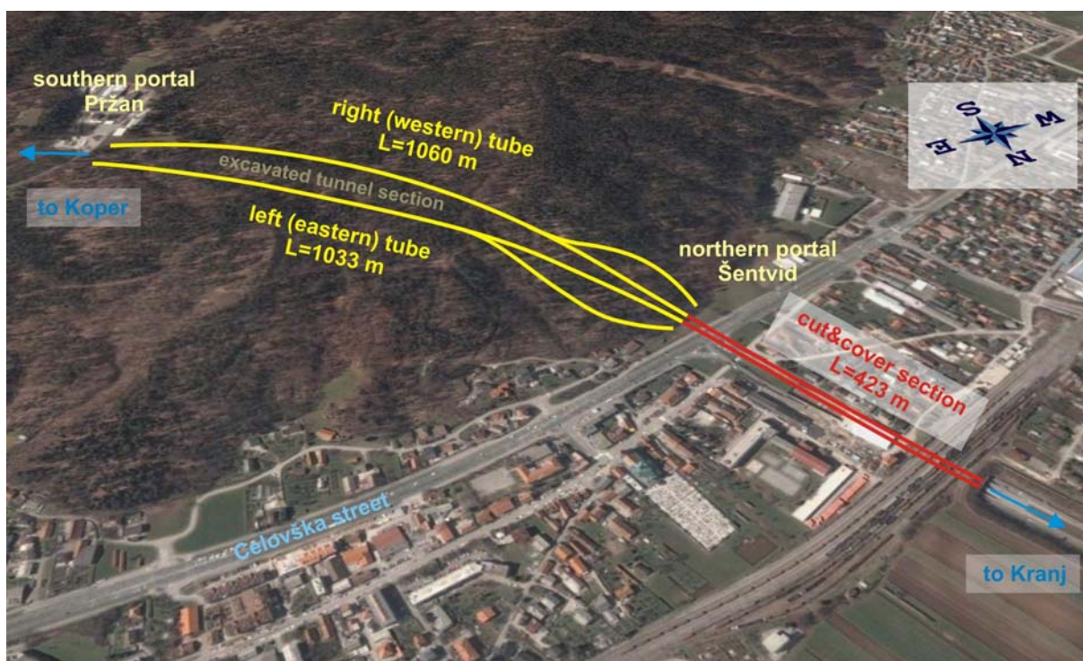
Figure 2-6. Layout of the Šentvid tunnel.
