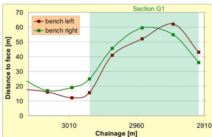
Figure 4-19. Distance between the bench excavation face and the measuring section when the latter can be considered as stabilised in the area of section G1 in the eastern tube of the Golovec tunnel.
