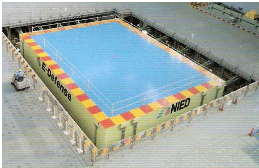
Slika 29: Potresna miza E-Defense v laboratoriju NIED
