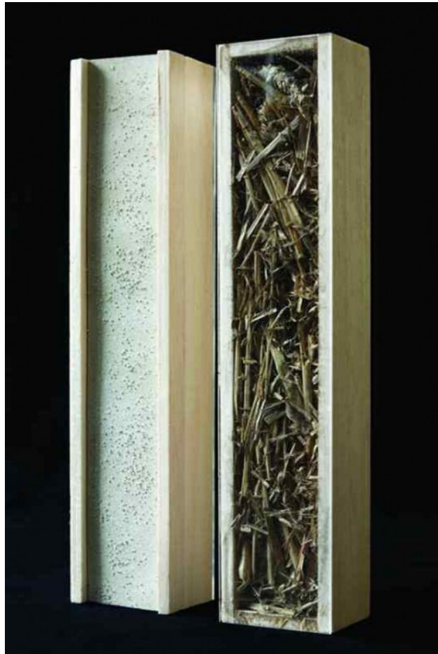
Slika 28: Panel, uporabljen pri gradnji (vir: http://inhabitat.com/work-begins-on-the-uks-largest-prefabricated-strawbale-building )
