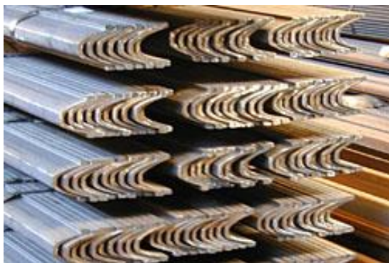
Slika 18: TH-jekleni loki Vir: http://www.dywidag.com/products/tunneling
