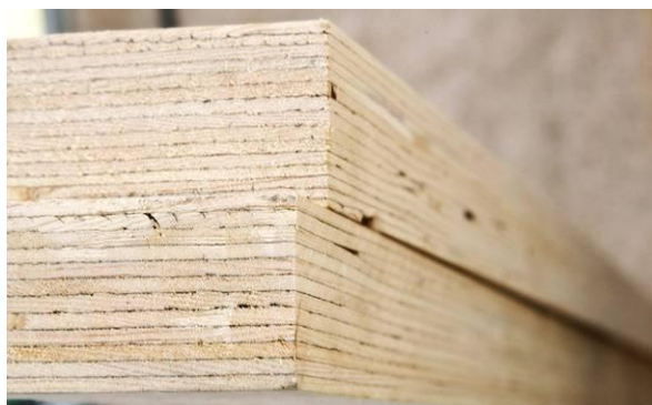
Slika 2.5: LVL Ultrallam ® ( http://www.taittimber.com.au )
