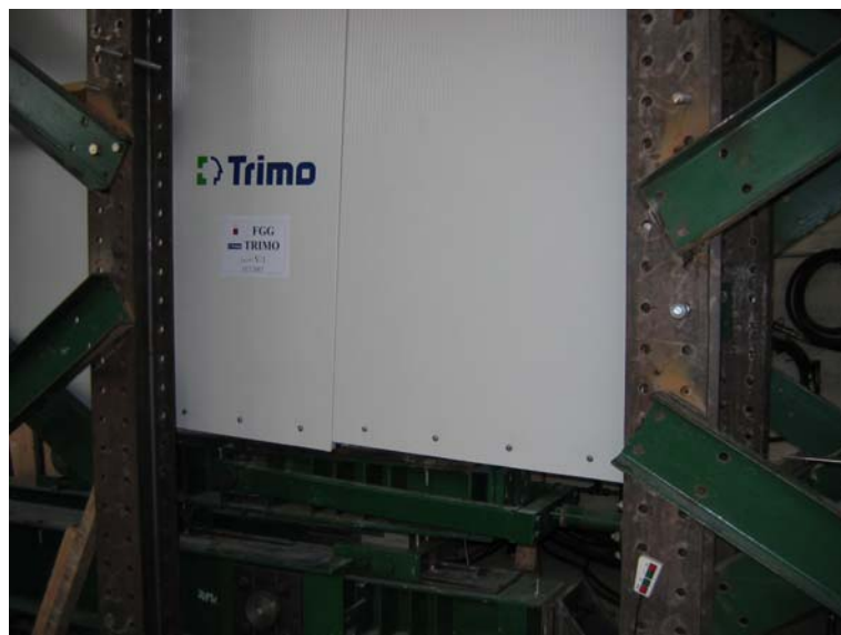
Slika B.29: Test V/1, omejen zdrs med posameznimi paneli (enostransko šivan spoj) Figure B.29: Test V/1, limited slide between sandwich panels
