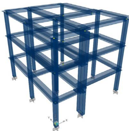
Slika 5.9: Matematični model v programu SAP2000 Figure 5.9: Mathematical model of the structure SPEAR (SAP2000)
