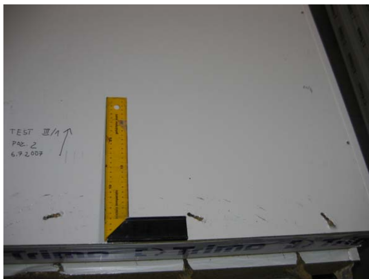
Slika B.11: Pretrg notranje pločevine sredinskega panela Figure B.11: The tear of the inner steel sheeting of the central sandwich panel
