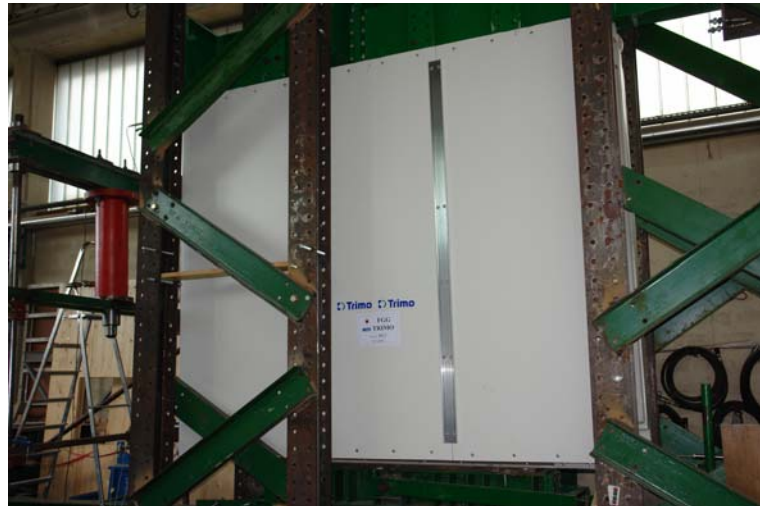
Slika B.18: Test III/3, brez zdrsa med posameznimi paneli Figure B.18: Test III/3, without slide between sandwich panels
