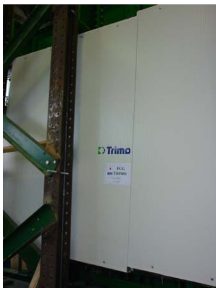
Slika 2.32: Zdrs med paneli Figure 2.32: Slide of the two panels
