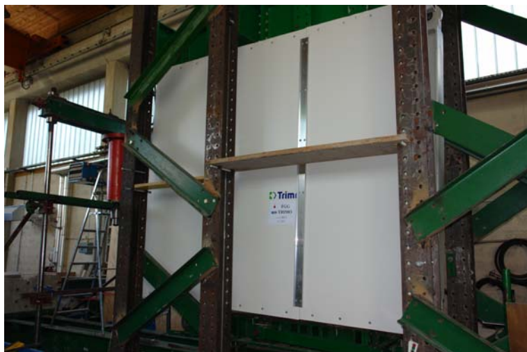
Slika B.10: Test III/1, brez zdrsa med posameznimi paneli Figure B.10: Test III/1, without slide between sandwich panels
