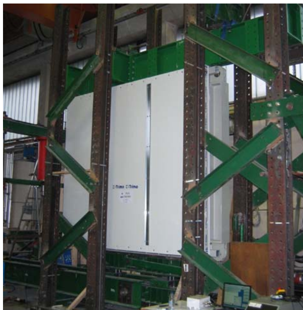
Slika 2.23: Preizkušanec III/1 s šivanim spojem in z štirimi vijaki med posameznim panelom in lego Figure 2.23: The specimen III/1 with seam connections and four bolts per meter
