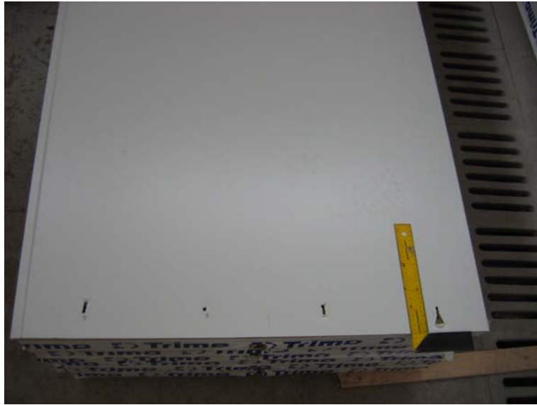
Slika B.7: Pretrg pločevine na notranjem robu panela Figure B.7: The tear of the inner steel sheeting of the sandwich panel
